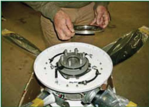
*Installing the slip ring.*
