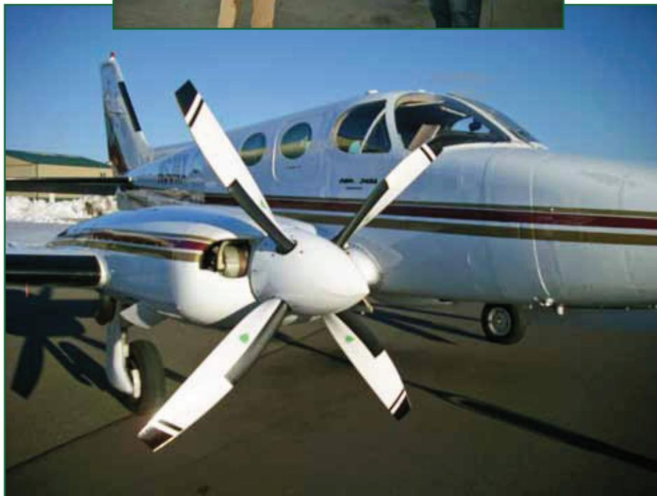
*The addition of MT composite props made a superb 340A even better. Check out these before and after shots. (Above) That's me on the right and Larry Schlasinger from Flight Resource on the left.*
